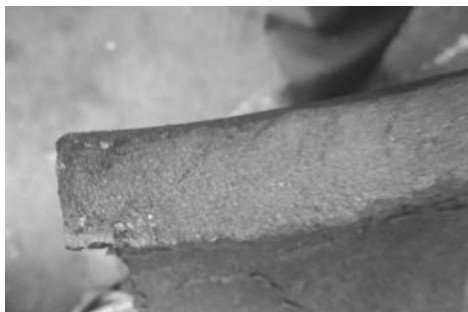
图5 球铁管管壁断口情况 Fig. 5 Fracture of ductile iron pipe wall
