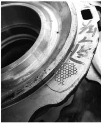
图24 过滤片破损夹杂 Fig. 24 Inclusion for strainer core broken
