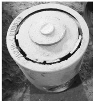
图20 漂芯 Fig. 20 Core raised
