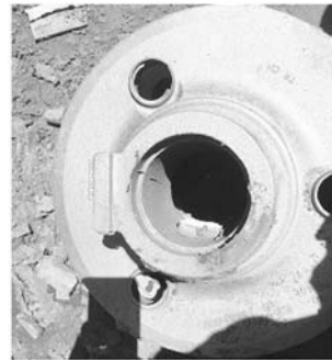
图2 浇冒口残留多肉 Fig. 2 Metallic projections at casting head
