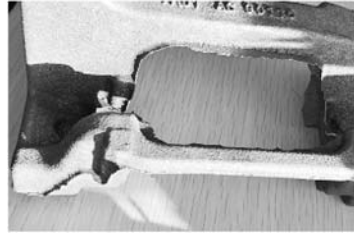
图1 飞翅 Fig. 1 Joint flash
