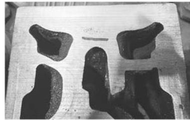
图8 缩松 Fig. 8 Dispersed shrinkage
