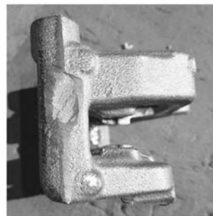
图19 浇冒口带肉 Fig. 19 Broken casting at gate
