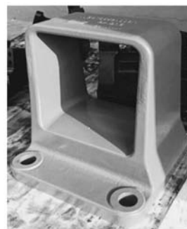
图1 150 t重卡ADI板簧支架 Fig. 1 ADI plate spring support for the 150 t heavy trucks
