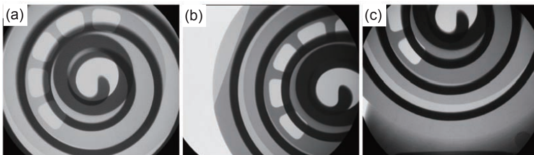
Fig. 19: X-ray detection of the central (a), left (b), and bottom (c) part of the scroll casting fabricated by SSSC process
